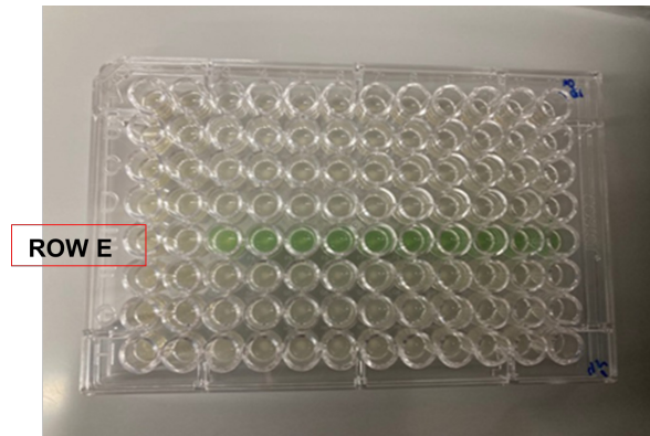
ABOVE: The 96-well plate with Mueller-Hinton Broth supplement added to columns 2-12 and chlorine solution (sodium hypochlorite solution, 12%) added to columns 1 & 2. Serial dilutions from columns 2-11. *Column 12 left without chlorine disinfectant (growth control). Bacterial suspension added to each well (final concentration 7.5 \times 10^5 CFU/mL). *ROW E demonstrates strong biofilm potential (in response to chlorine exposure) of pathogenic, multidrug-resistant P. aeruginosa strain cultured from chlorine-treated water sample. 11
